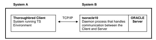
In the above figure the information is sent over the network to the server system. Once the requests reach the Server Process it creates SQL statements that are interpreted by the server system. The results are then passed back to the client through the Server Process.
